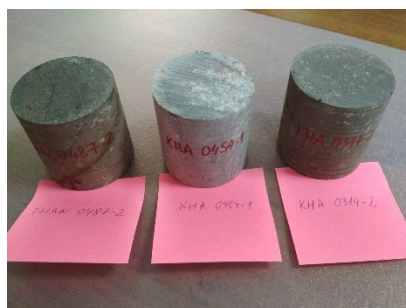
Fig.1. Extracted core specimens of the depth of 477 m, 464 m and 314 m from the two boreholes PHAN and KHA.
